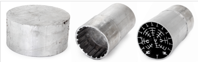
1, Put an aluminium ingot into hydropress, getting a primary lamp model.
