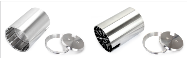
2. Lathe the lamp model, getting a delicate lamp body.
