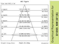
Note: The Curves indicate the illuminated area and the average illumination when the luminaire is at different distance.
