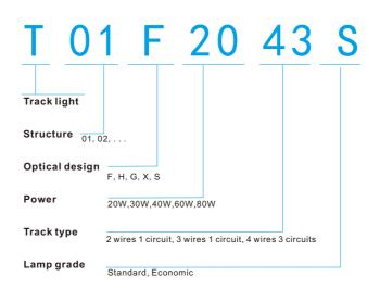
Available track holder: 2 wires 1 circuit, 3 wires 1 circuit and 4 wires 3 circuits.
